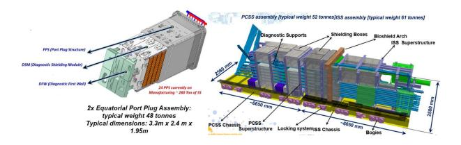
Figure 1. Typical integrated diagnostic port inside ITER infrastructure: left – inside vacuum (port plug); right – outside vacuum (interspace and port cell structures).
