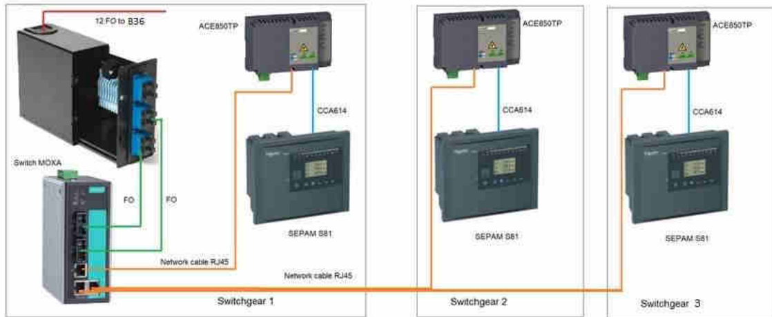
Overview of the sepam architecture (22kV+15kV)
