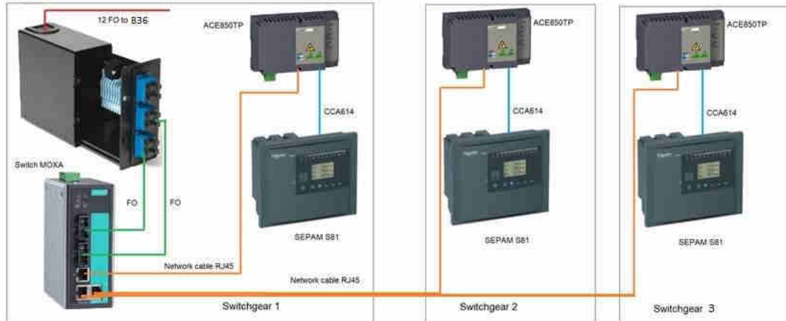
Overview of the sepam architecture (22kV+15kV)
